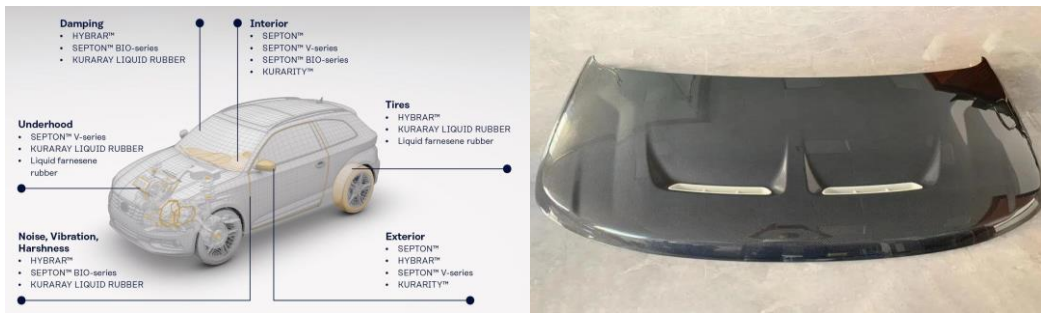
Fig. 2. Parts that can be manufactured from automotive polymers [23].
