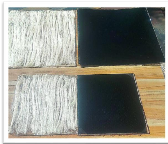
Fig. 6. Carbon fiber and palm fiber after pouring into the mold.
