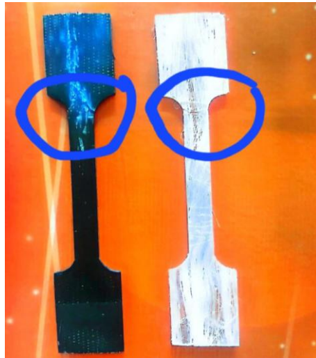
Fig. 9. Tensile test specimen after applied force and fracture.
