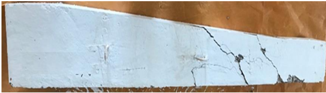
Fig. 14. Crack patterns of beam B300-8-L.
