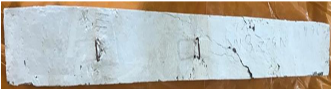
Fig. 15. Crack patterns of beam B225-8-L.
