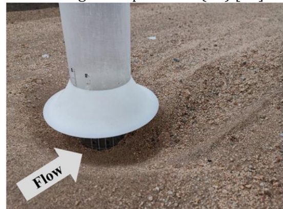
Fig. 4. Local scour formation after running the experiment (C1) [52].
