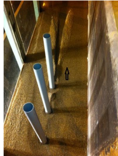
Fig. 4. Local scour formation after running the experiment (C1) [52].
